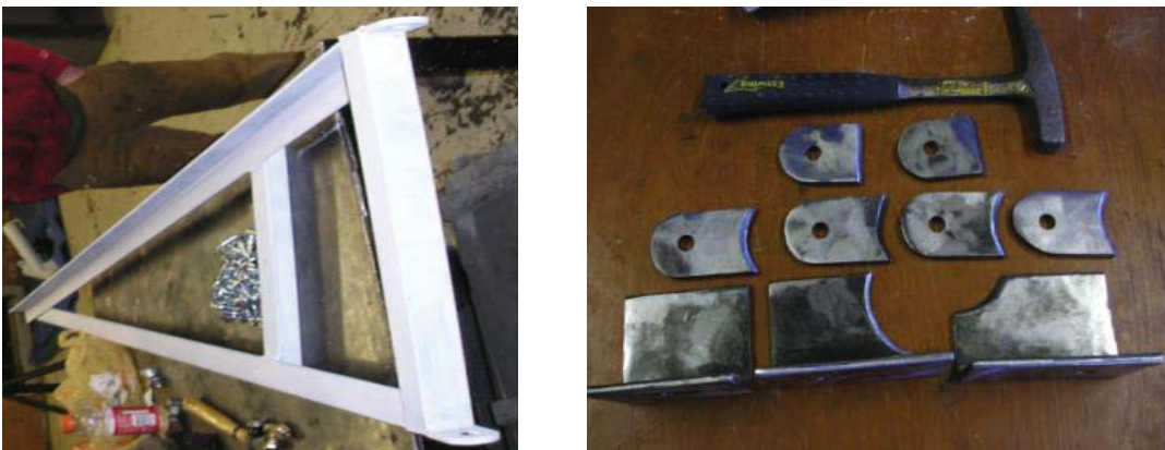
Figure 4: Initial Steel Assembly. Yaw bearing tube (vertical pipe on left) mounted to horizontal alternator mount. Trailer hub shown. Jacking screws shown in lower right. (left). Wood Blades (left of right image), Circular mounting disc (middle of right image), Triangular blade mount (right of right image) Native weather resistant wood OR fiberglass blades (mold created at KIST from a blade carving). The 'triangle' and the circular disc to the right sandwich the blades together at the base, where it is mounted to the hub.
