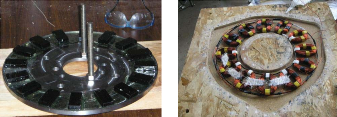
Figure 3: Completed tail frame assembly (left). Tail lugs on top two rows and Stator Mounts on bottom row (right).
