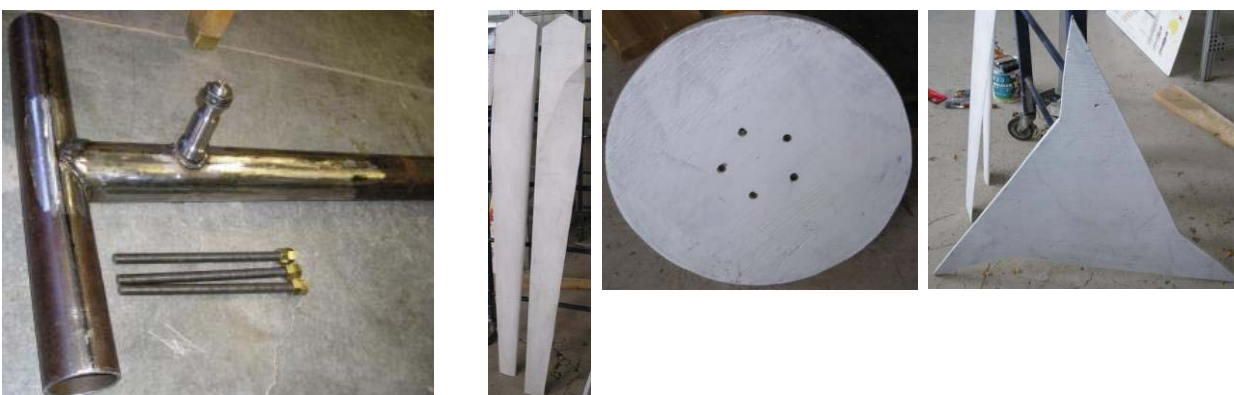
Figure 4: Initial Steel Assembly. Yaw bearing tube (vertical pipe on left) mounted to horizontal alternator mount. Trailer hub shown. Jacking screws shown in lower right. (left). Wood Blades (left of right image), Circular mounting disc (middle of right image), Triangular blade mount (right of right image) Native weather resistant wood OR fiberglass blades (mold created at KIST from a blade carving). The 'triangle' and the circular disc to the right sandwich the blades together at the base, where it is mounted to the hub.
